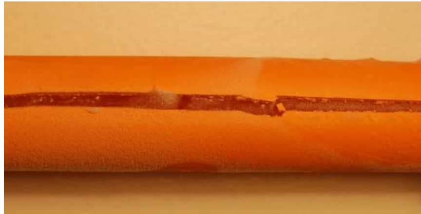
Figure 7. Picture of frozen CPVC pipe.
