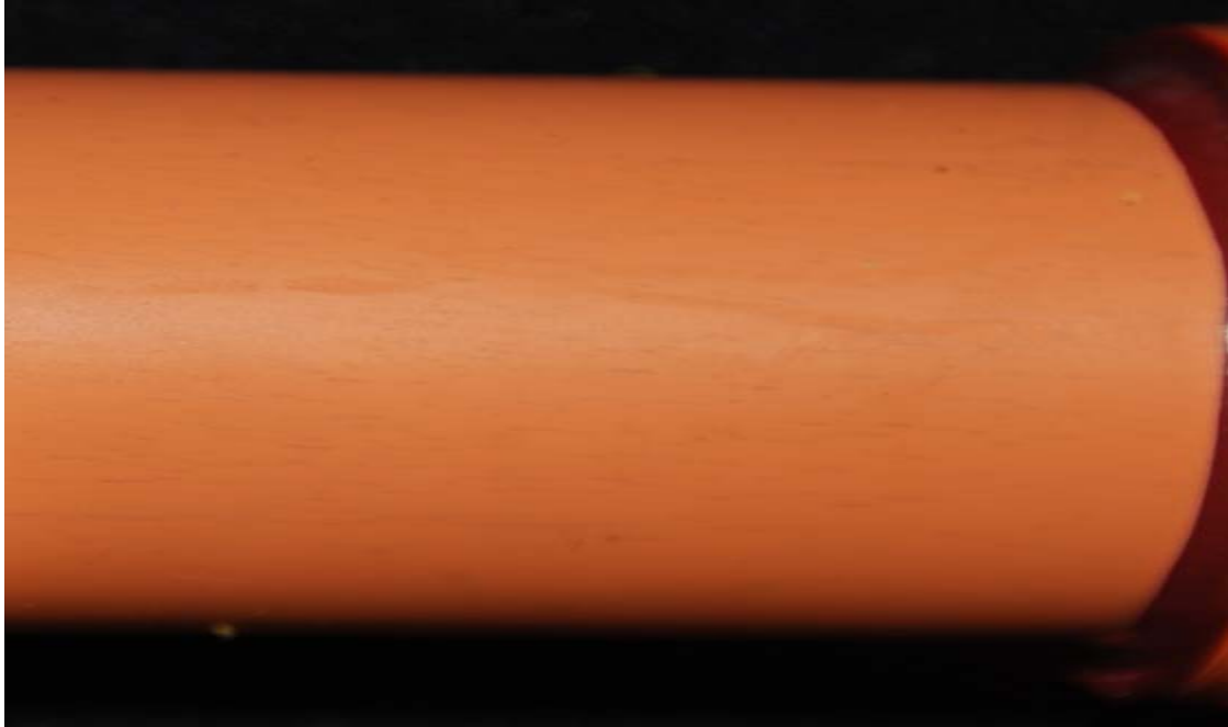
Figure 17. Extensive surface crazing of outside pipe wall.
