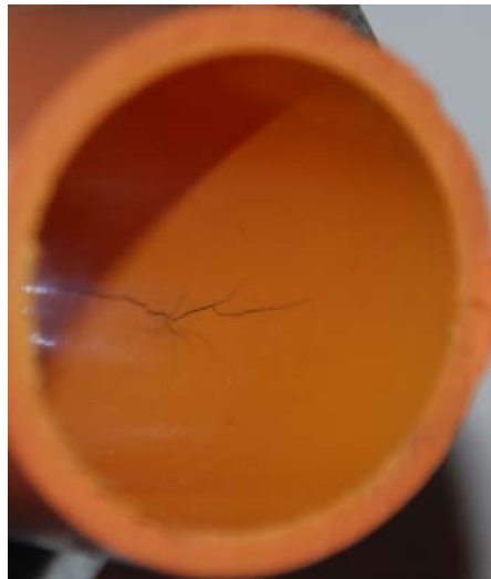
Figure 1. Formation of a stress-crack on the inside of a CPVC fire sprinkler pipe at a point where a tight-fitting clamp was used.
